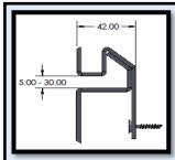
(Artisan Panel) (ART-PAN) 42mm (Maxi panel) for materials 1mm to 3mm thick
