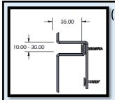
(Artisan Panel) (ART-PAN) 35mm (Structural panel) for materials 1mm to 3mm +
